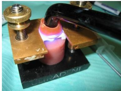
Figure 2. Jig in which the composite is applied to conduct the test.
